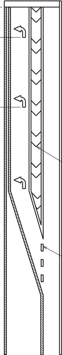
Chevron markings shall be used for offsets greater than 6'. Follow crosshatching guidelines shown in Sepia 046 for dimensions and spacing.
