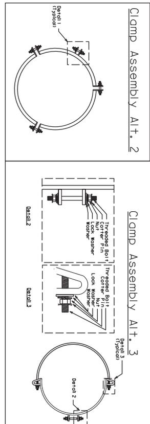
**CLAMP/CLEVIS-** ASTM A36 (GRADE 36)/ASTM A572 (GRADE 50)
